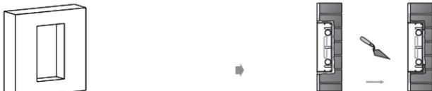
According to the position of the cable cut a square hole in the wall (height\*width\*depth=180\*101\*50 mm). Note: The size of the hole should be a little larger than recommended value that it can accommodate all needed cables.
