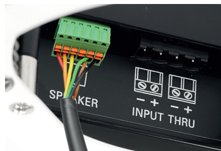
6-pole connection with screw type terminals
