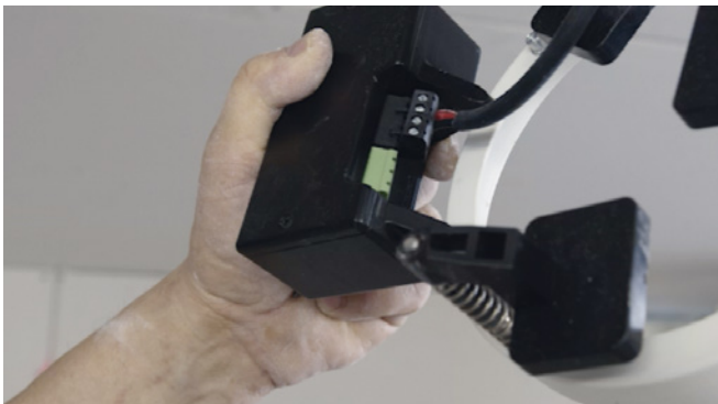
Insert terminal at input of crossover.
